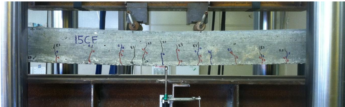
Figure C20. Flexure test on beam – Mix 15CF
