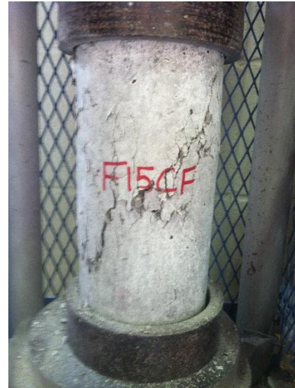
Figure A42. Mix F15CF - 28-day Compressive Failure
