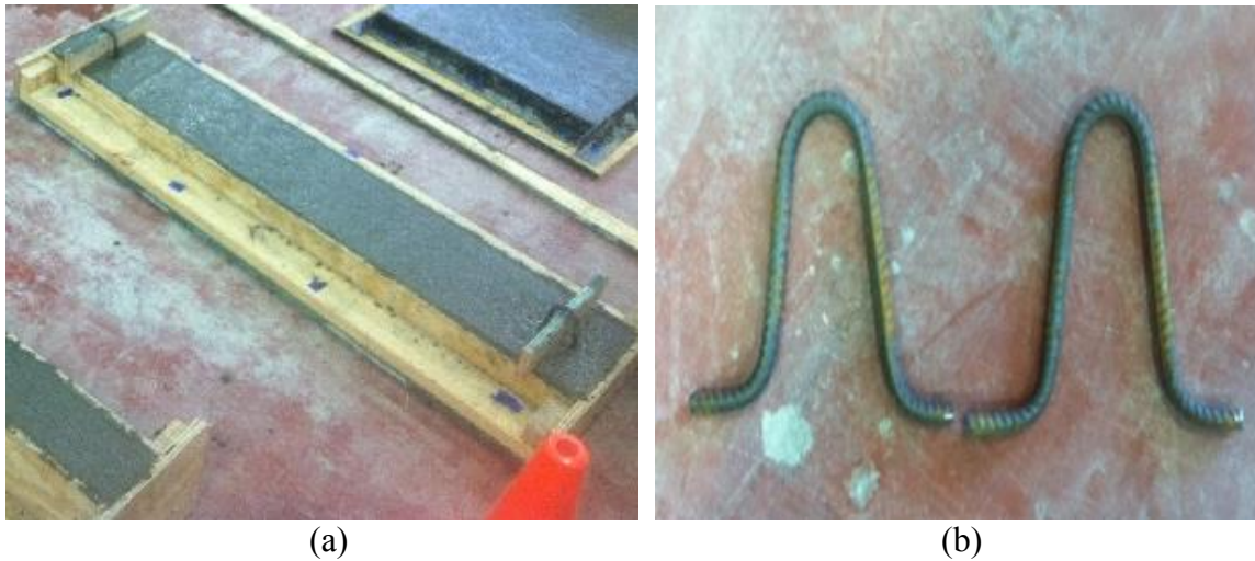
Figure 8. (a) Finished flexure beam and (b) Hooks placed in beam ends
