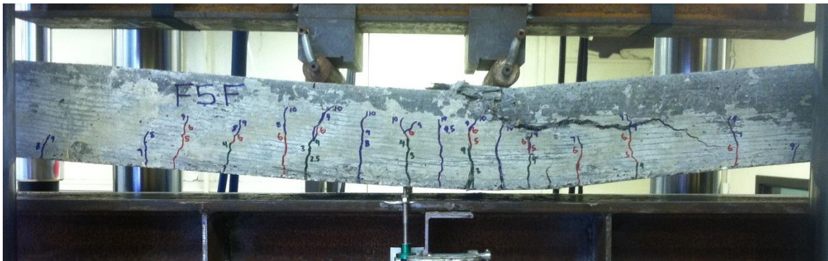
Figure C28. Flexure test on beam – Mix F5F
