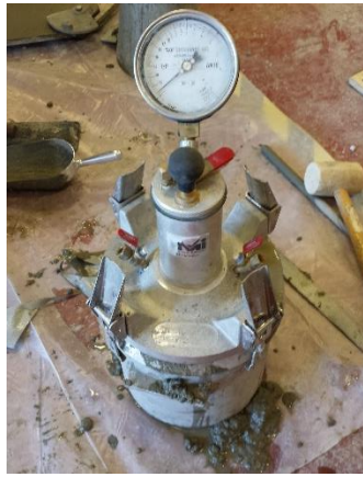
Figure 11. Air content test setup
