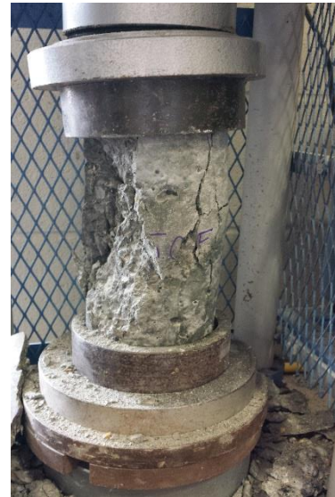
Figure A8. Mix 5CF - 28-day Compressive Failure
