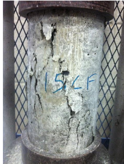
Figure A20. Mix 15CF - 28-day Compressive Failure
