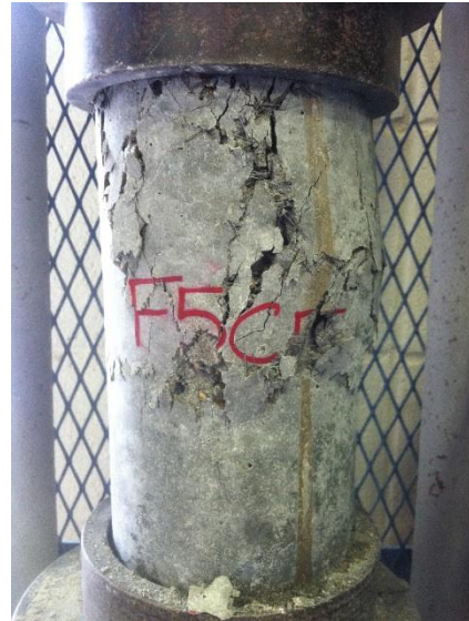
Figure A30. Mix F5CF - 28-day Compressive Failure
