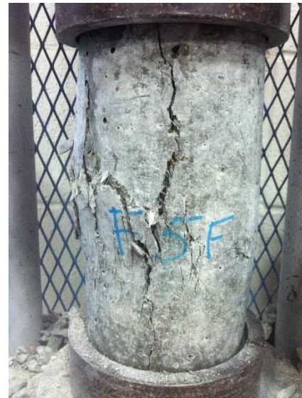
Figure A28. Mix F5F - 28-day Compressive Failure
