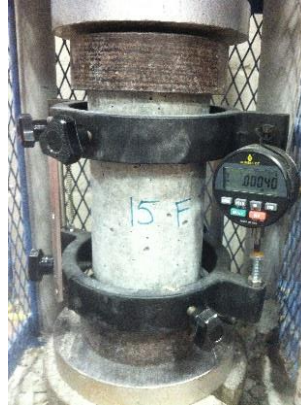
Figure 14. Modulus test setup
