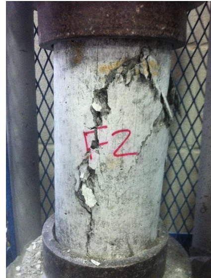
Figure A44. Mix F2 - 28-day Compressive Failure
