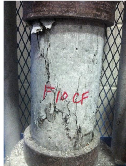
Figure A36. Mix F10CF - 28-day Compressive Failure
