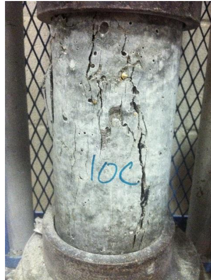
Figure A10. Mix 10C - 28-day Compressive Failure
