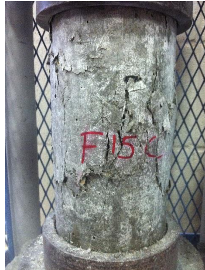
Figure A38. Mix F15C - 28-day Compressive Failure
