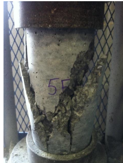
Figure A6. Mix 5F - 28-day Compressive Failure
