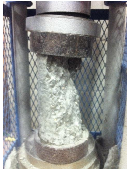
Figure A2. Mix PL1 - 28-day Compressive Failure
