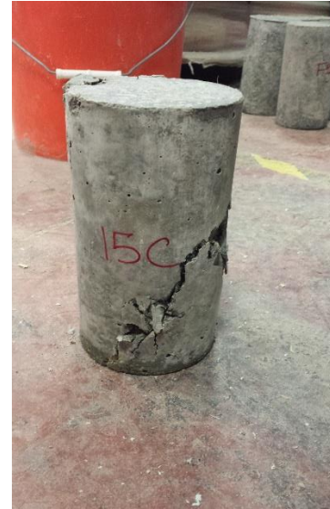
Figure A16. Mix 15C - 28-day Compressive Failure
