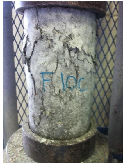
Figure A32. Mix F10C - 28-day Compressive Failure
