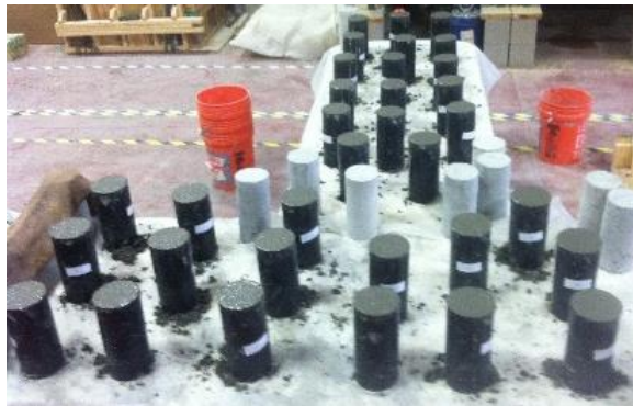
Figure 7. Fresh concrete cylinders
