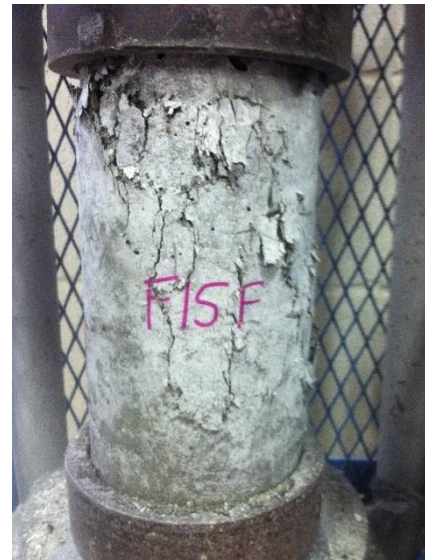
Figure A40. Mix F15F - 28-day Compressive Failure
