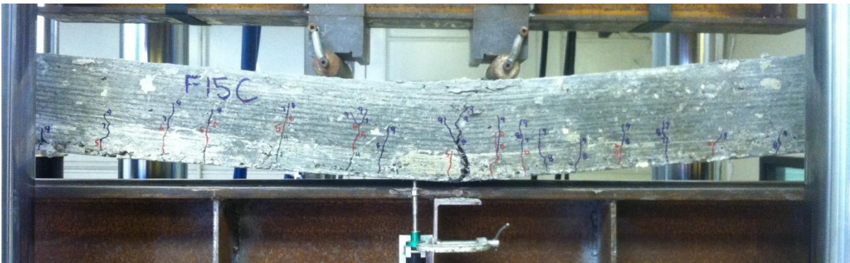
Figure C38. Flexure test on beam – Mix F15C
