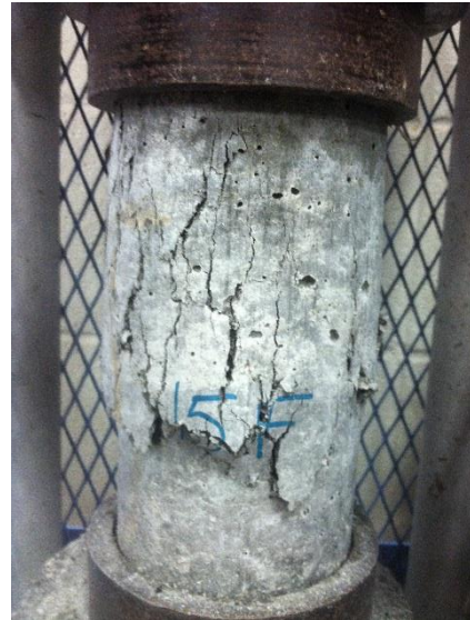
Figure A18. Mix 15F - 28-day Compressive Failure
