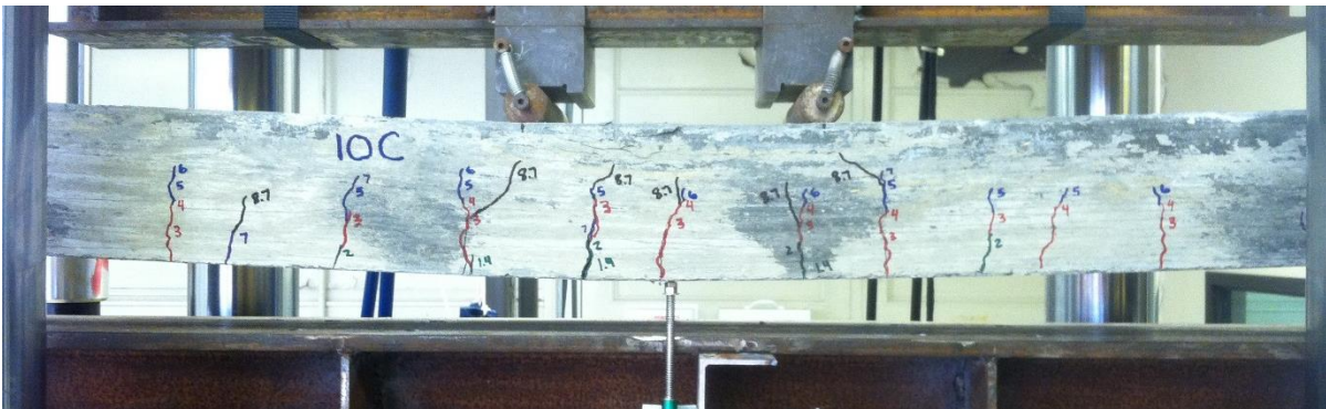
Figure C10. Flexure test on beam – Mix 10C
