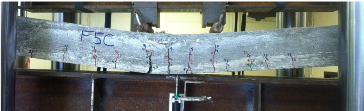
Figure C26. Flexure test on beam – Mix F5C
