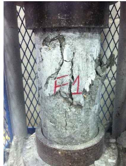
Figure A24. Mix F1 - 28-day Compressive Failure
