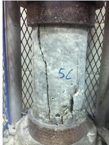
Figure A4. Mix 5C - 28-day Compressive Failure
