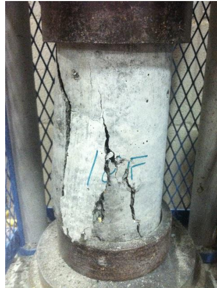
Figure A12. Mix 10F - 28-day Compressive Failure
