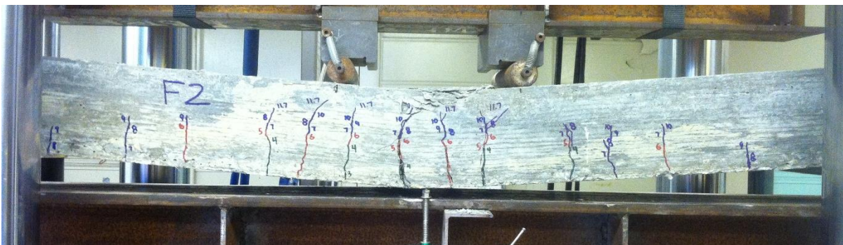
Figure C44. Flexure test on beam – Mix F2
