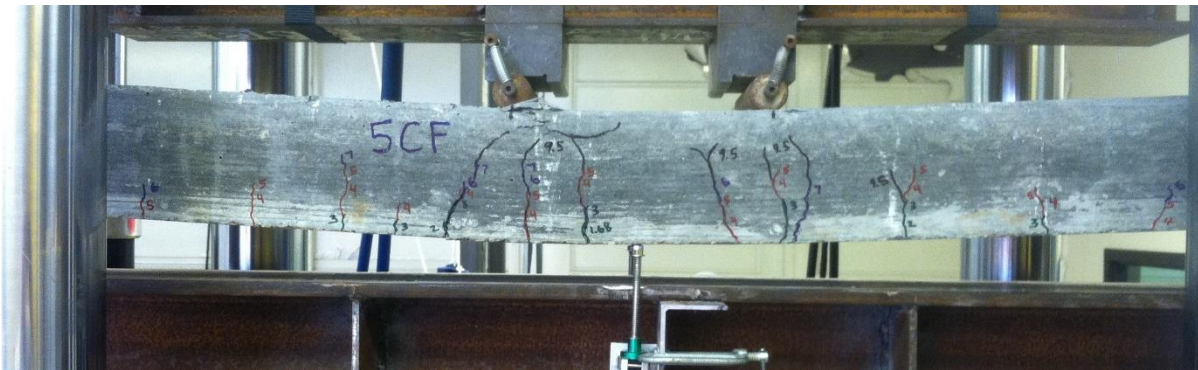
Figure C8. Flexure test on beam – Mix 5CF
