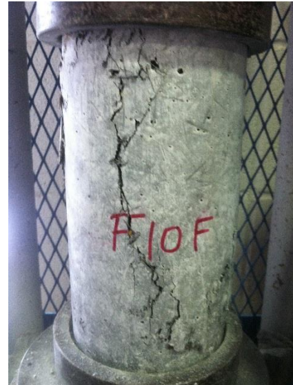
Figure A34. Mix F10F - 28-day Compressive Failure
