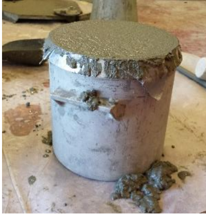
Figure 10. Unit weight container filled with fresh concrete
