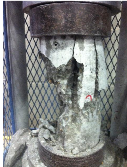
Figure A22. Mix PL2 - 28-day Compressive Failure
