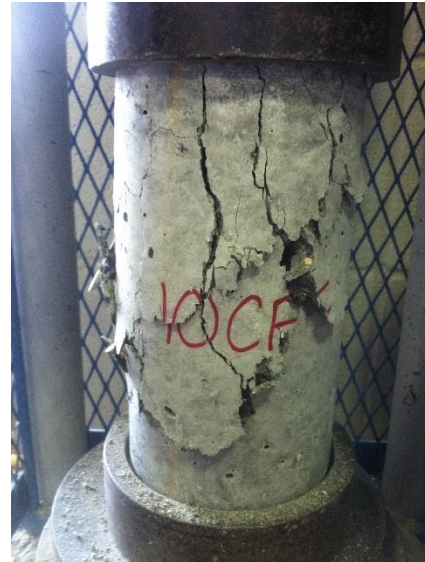
Figure A14. Mix 10CF - 28-day Compressive Failure
