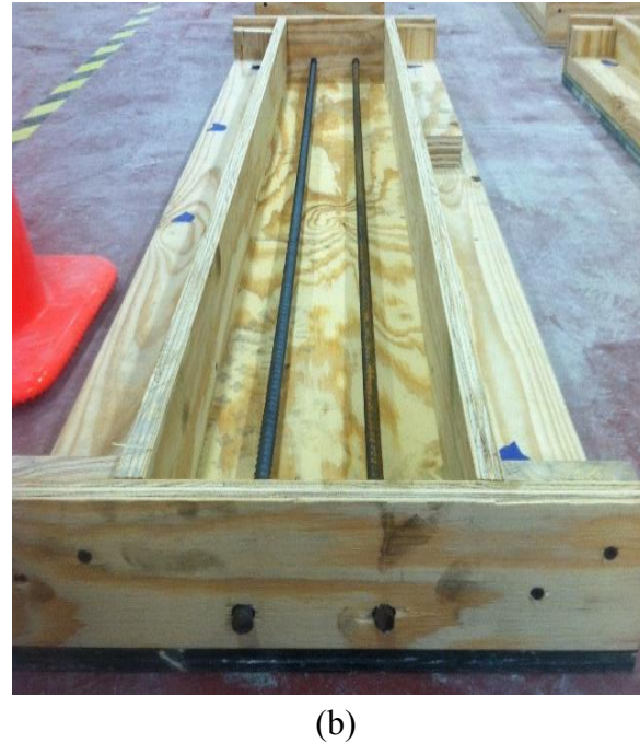
Figure 5. (a) End piece on flexure beam formwork and (b) Flexure beam formwork
