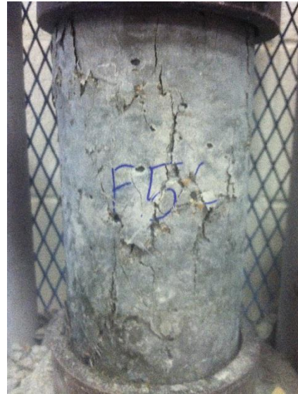
Figure A26. Mix F5C - 28-day Compressive Failure
